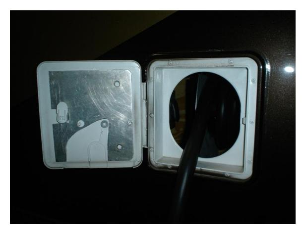
Now when the access door is closed it will stay closed and there will be less chance of rain entering the power cord compartment. With the new driver side cap rails and new drip rail with a down spout pouring water down the coach wall directly over the access door this modification was needed now more than before the rails and down spout were added.
