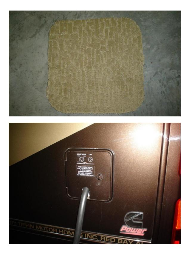
While working on the power cord reel, I found the outside access door which is plastic would bend or warp over time allowing the door to pop open or just be hard to close and keep closed at times.
